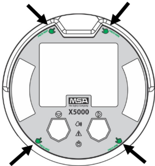
Figure 24 Highlighted Areas Show Where to Press when Replacing a Board Stack
