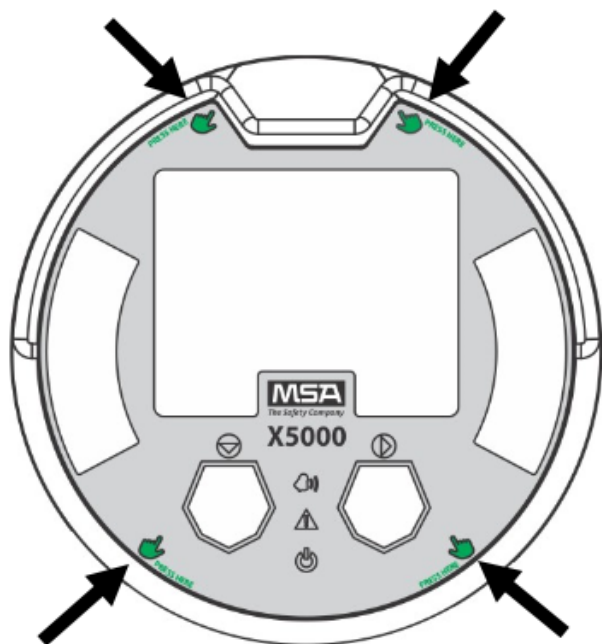
Figure 10 Highlighted Areas Show Where to Press when Replacing a Board Stack
